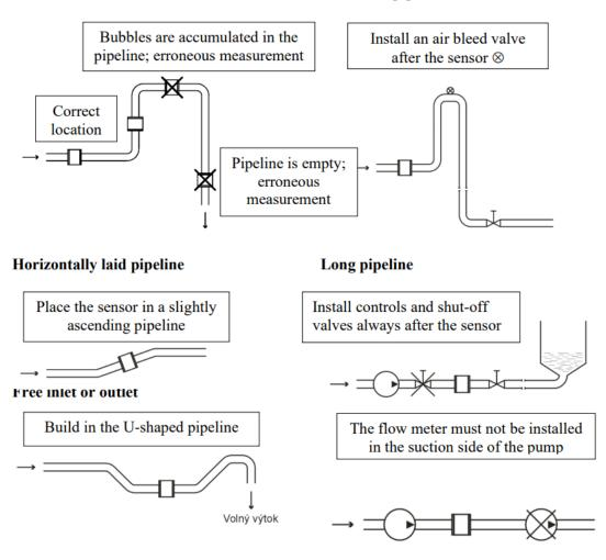
The flow of liquid flow in the flow sensor should be steady and free of whirling. For this reason, straight sections of pipeline with the same ID as that of the flow meter before and after the flow sensor (with permissible deviation of +5%). Recommended minimum length of straight sections is 5×d before the flow sensor and 3×d after the flow sensor where d is the inside diameter of the meter in millimetres.
