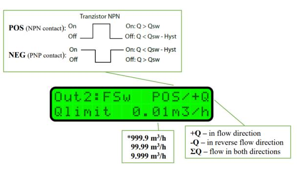
\*Qlimit - the number of decimals is given by the DN of the given meter and cannot be changed.
