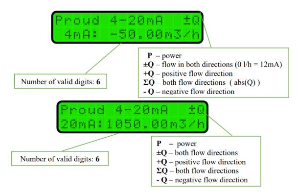
The current loop can be calibrated by changing the Posun (offset) value.
