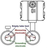
Every time when the empty tube testing electrode is not covered with a liquid for 5s at least, the flow meter will display the "Empty tube" status, and if it is necessary, it sends out an error message and stops taking measurement. The measurement accuracy is maintained in this way. Once the electrode is covered with the liquid again, the error message disappears and the flow meter starts taking measurement again.
