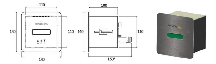
\*The necessary mounting depth, including the cable connector from the flow sensor is 200mm
