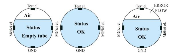
2) Incorrect installation (evaluation unit is positioned diagonally, Empty test - ON)
