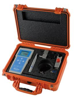
Use the 5-button keypad and menu system to set up the flowmeter by entering the pipe material, diameter and wall thickness. The PTFM 1.0 calculates the transducer separation distance and mounting method automatically.
