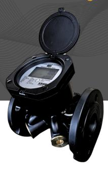
Kimans Hydrasonic i-UWM is designed with multi path sensors ultrasonic technology to measure the water flow even in low flow rates. It is build on the principle of transit time for accurate flow measurement.
