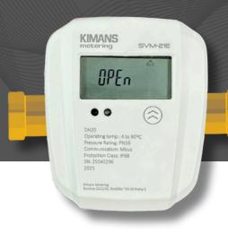
The SVM 21E smart valves are battery-powered open/close valves designed for remote flow disconnection and operate using the M-Bus protocol. They feature a manual override isolation function, integrated software for monitoring, control, and error reporting, and are encased in an IP68-rated protective housing for durability.
