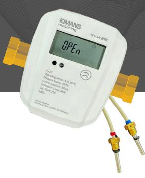
The SVM-21E smart valves are battery-powered, M-Bus-operated open/close valves for remote flow disconnection, featuring manual override, integrated monitoring/control software, and error reporting. Housed in an IP68-rated enclosure, they include temperature sensors to enable  $\Delta T$  (delta-T) control.
